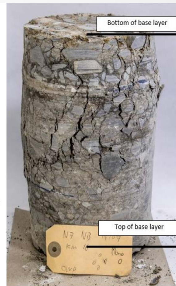
Figure 4.27: Core after triaxial testing (NB km 16 tested at 0 kPa)
